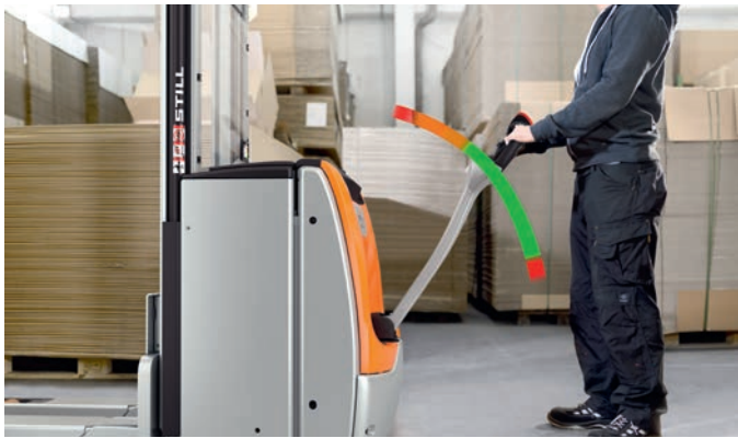
Safety in production: depending on the tiller angle, the speed is automatically adapted to the distance between the operator and the truck
