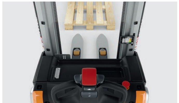
STILL free view mast always ensures the best view of the tips of the forks
